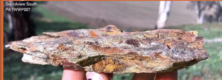
Highly sheared limonitic gold bearing rock from 35g/t Au sample site
