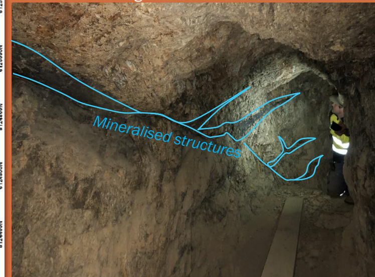
High grade flat lying mineralised structures which historic miners targeted in adit
